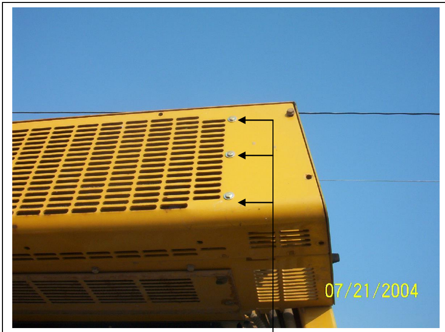
Condenser mounting bolts
