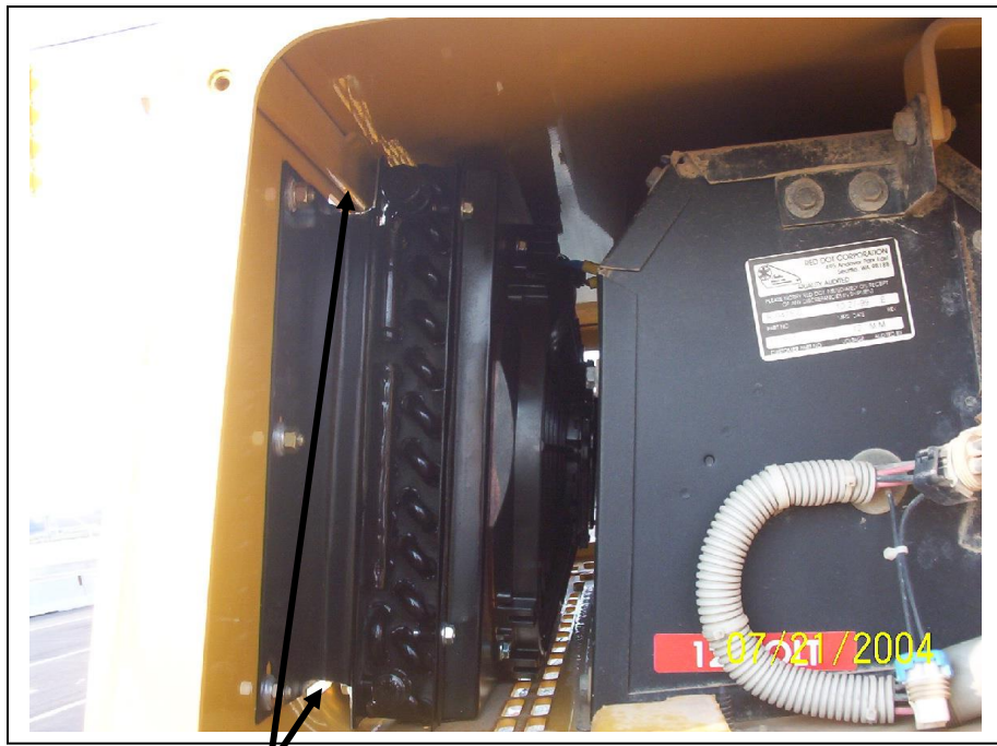
Seal air gaps with foam or tar tape.
